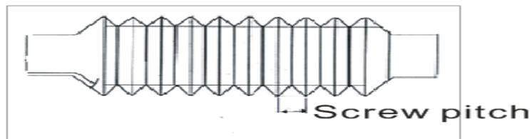
Screw pitch(above picture): The distance that the nut moves when the ball screw makes one rotation.
