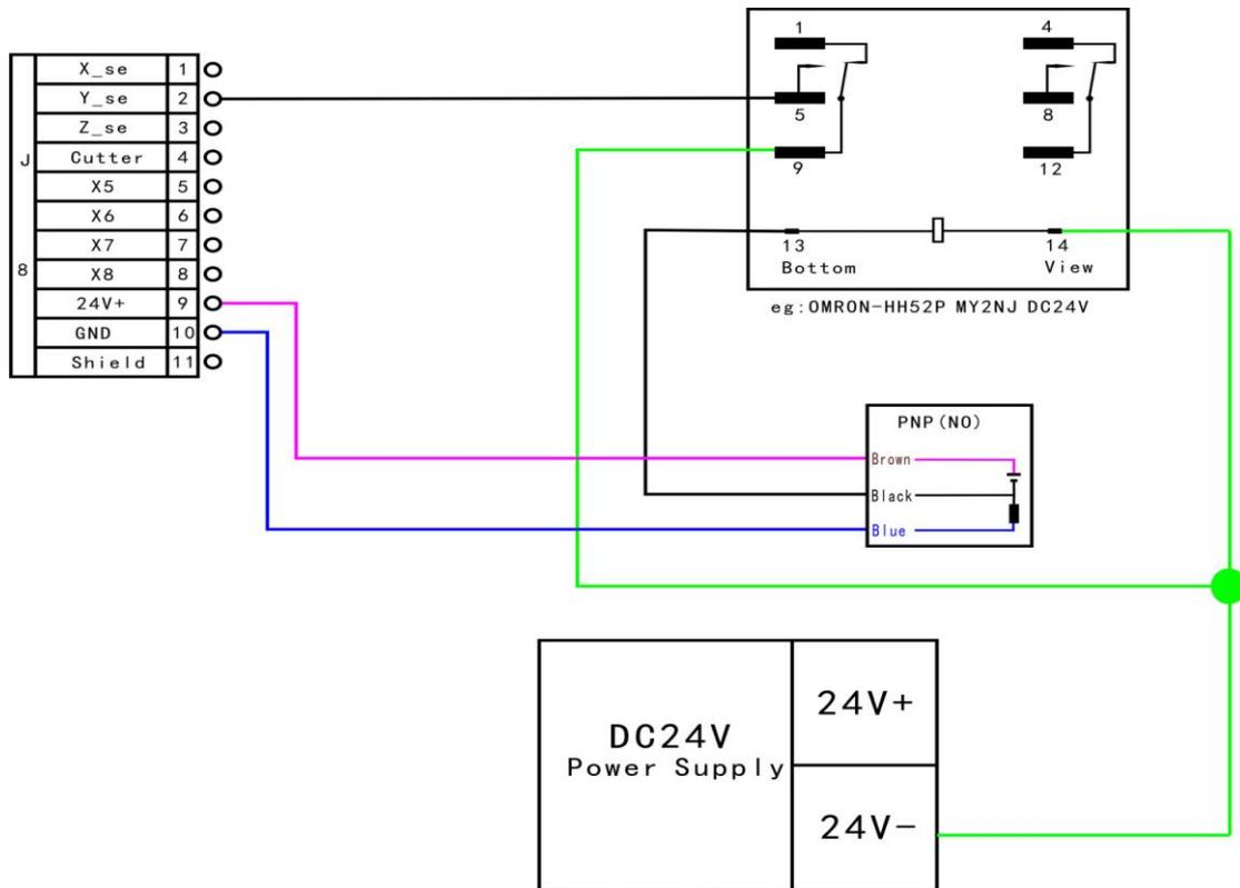
2 Tool-setting input: Tool-setting detecting wiring:
