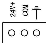
Fig. 2-2 Pin definition of +24V power input interface
