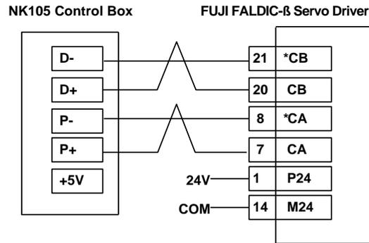
Fig. 10-8 Wiring diagram of NK105 and FUJI FALDIC-β servo driver
