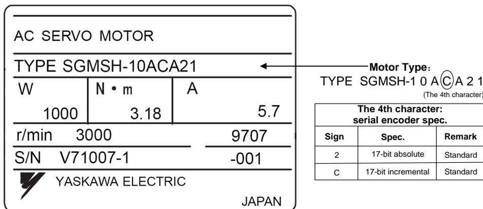
Fig. 5-2 Name plate of servo motor-encoder resolution
