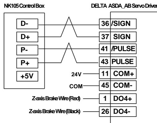
Fig. 10-5 Wiring diagram of NK105 and DELTA ASDA\_AB servo driver
