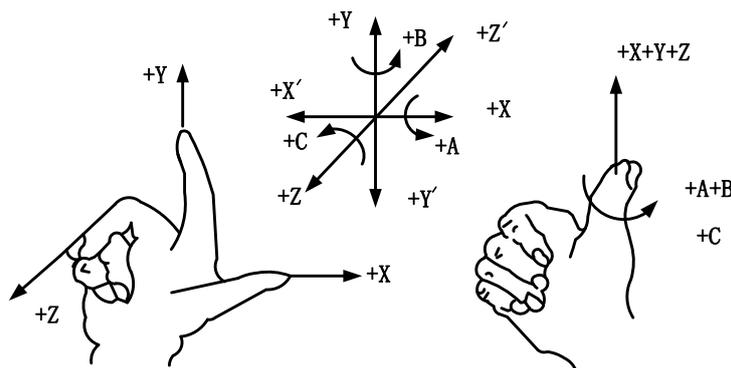
Fig. 3-1 A coordinate system conforming to right-hand rule
