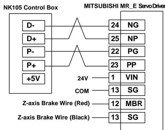
Fig. 10-7 Wiring diagram of NK105 and MITSUBISHI MR-E servo driver
