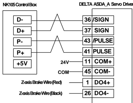
Fig. 10-4 Wiring diagram of NK105 and DELTA ASDA\_A servo driver
