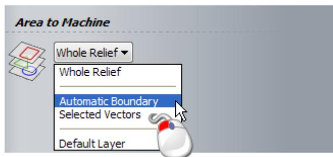
A boundary vector is calculated from the tool's geometry and is drawn on the currently active vector layer (see page 124).
