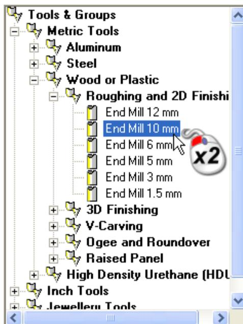
The **Tool Database** closes, and your selected tool's description is displayed on the control bar. For example, *End Mill 10 mm*. For further details on using the **Tool Database**, see Using the Tool Database (see page 263).
