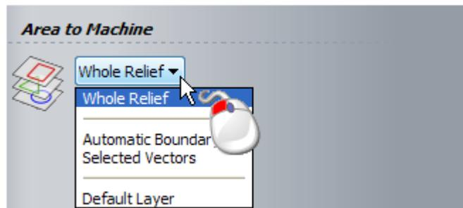
The **Machine Relief** panel's **Area To Machine** list box includes an additional option that enables you to machine as closely as possible to the composite relief above or below its base height using a chosen tool: **Automatic Boundary**.
